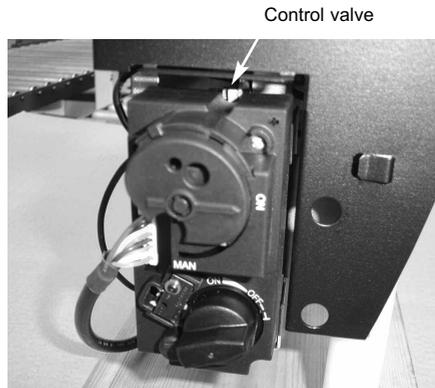
To re-fit the controls cover, locate in the slot and clip and fit back in position.
