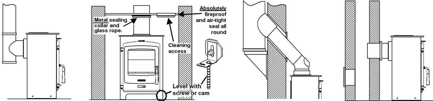
Rear outlet to top outlet by 'T' piece with cleaning door- the preferred method.
