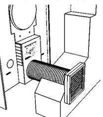
The Safety Air Supply kit, available as an extra, provides the correct fresh air for combustion and ventilation via a flexible tube from outside, without draughts across the room and meets the complete requirements of UK and RoI Building Regulations
