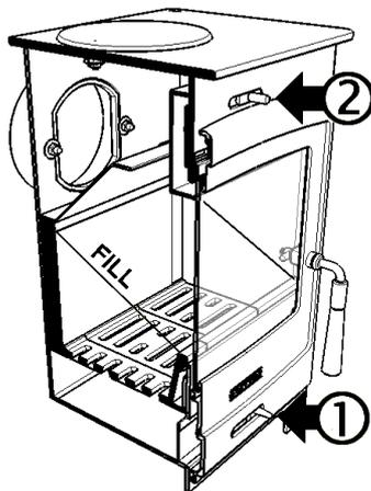
**FILLING:** Don't fill above the level shown in the diagram.
