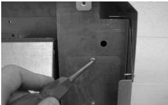
Fig. 13 Service Plate Removal
