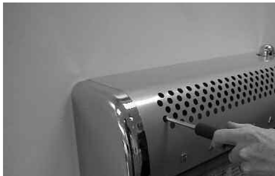
Fig. 10 Removing the Upper Outer Case Fixing Screws
