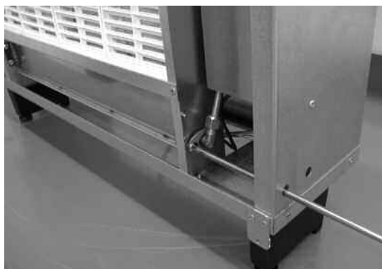
Fig. 11 Injector fixing bracket removal
