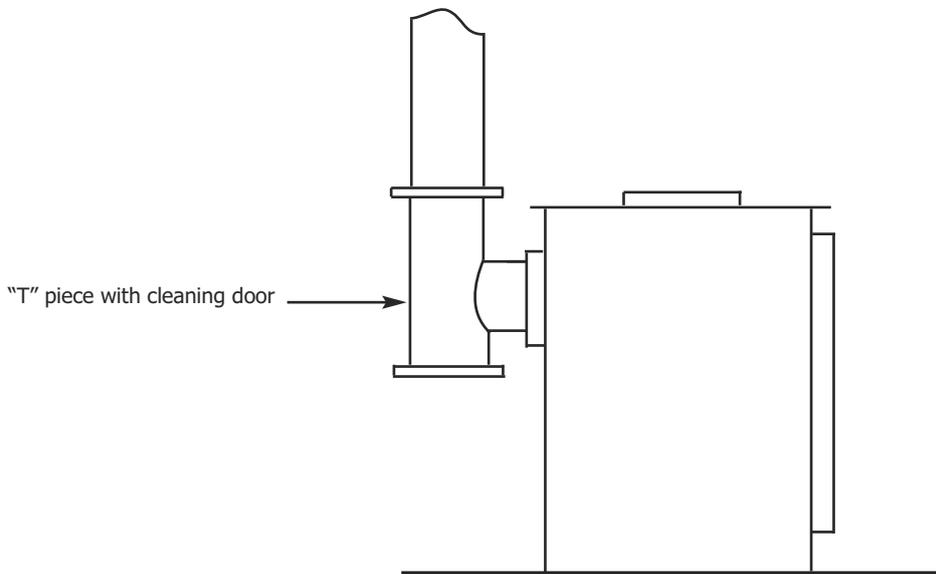
3.1.5 **IMPORTANT INFORMATION** - whichever method is used it is imperative that the route from the stove to the chimney terminal is completely air-tight, even very small air gaps can adversely affect the flue draught. Seal all joints with fireproof cement and / or heatproof rope. The entire construction should be made of durable fireproof materials.
